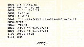
to the maximum or minimum values of y. We see an exponentially decaying sine wave. Also notice that both the x and y axes are labeled.
